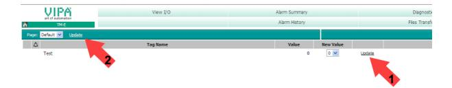
• If the new value is accepted by the CPU, so the communication between the TM and the CPU is secured.
